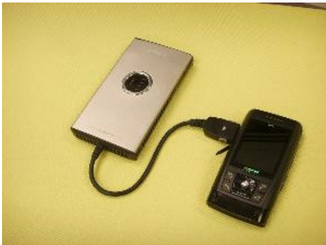
Fuel cell for charging mobile phones, MP3 players etc.
